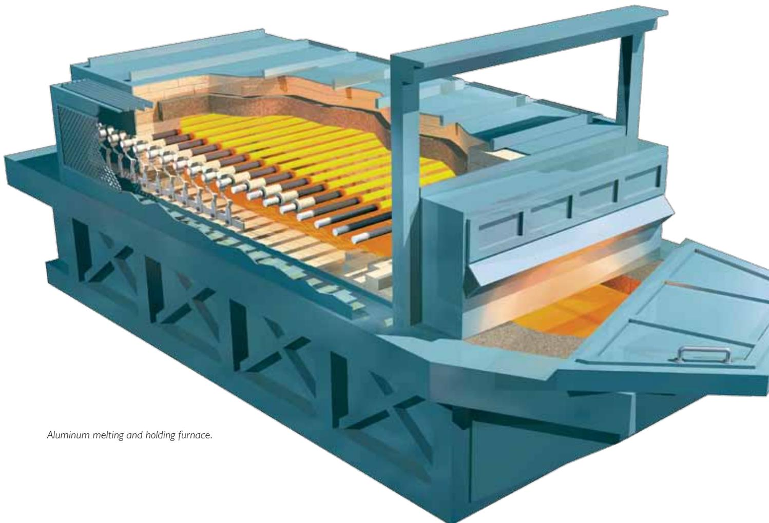
*Aluminum melting and holding furnace.*
